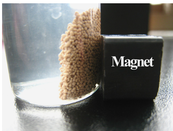
Fig. 4. Photograph of OMMT-Fe 3 O 4 @PSF microcapsules attracted by a conventional magnet.
